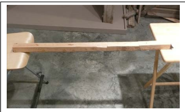
Fig. 14,15,16,17: Loose blocks epoxied to a 1.5in. carbon fibre tape in various arrangements from bent causing the blocks to spread and become quite flexible, to very rigid as the blocks come into contact and meet compressive forces. The stick spanning the chair and table will easily support a 200lb. person – the table is likely the weakest element. The three sticks at the right are: at the top a series of blocks with a tape below; the center stick has a 1.5in tape inserted into a saw cut; the bottom stick has the tape fully covering the face. With the tape on the side opposite the force, each will resist more strongly than a plain stick without the tape. Note: the loose blocks do not even need to be attached to the tape toward the center of the span – The tape requires a sound connection to the end blocks only. Attachment to several at the ends helps distribute the adhesive bond strength. A mechanical attachment to the end blocks would relieve the need for any adhesive.
