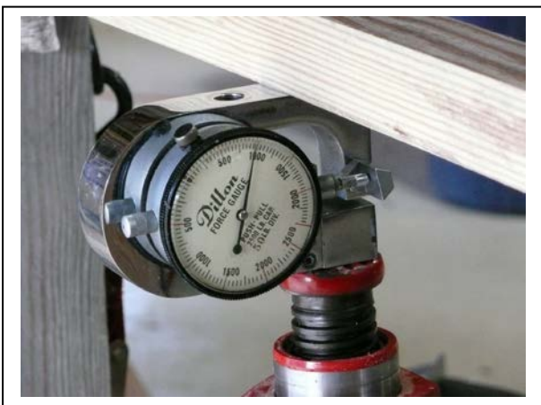
Fig. 20, 21: The initial jigs were quick, crude, but effective. The force gage was old and out of calibration but provided a good comparative analysis.
