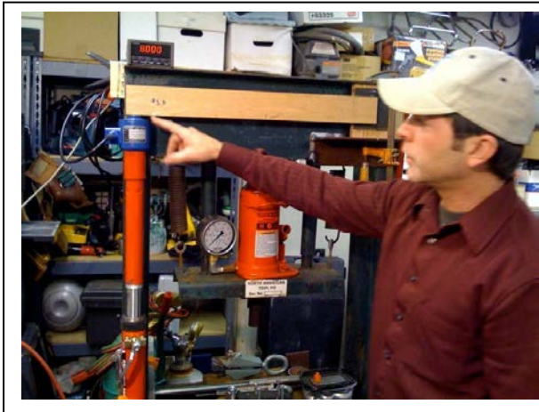
Fig. 22, 23: As the project progressed we got a little more sophisticated. This rig on the left is testing shear in torsion between the wood arm and the carbon fibre faced block seen just below the brim of the hat. The drawings on the right show the steps to making a carbon fibre core for a timber with a rotted center. Note the core will be filled with foam to reduce buckling.
