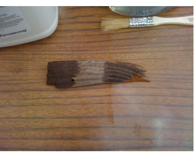
TWO DIFFERENT COMMERCIALLY AVAILABLE ACRYLICS WERE TESTED AT EACH END OF A SAMPLE BEFORE APPLYING EPOXY TO THE REAR.
