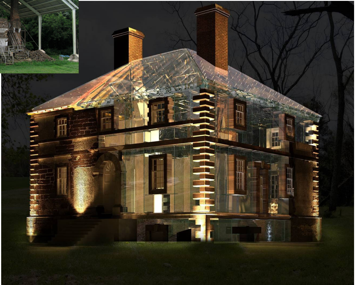
Innovative use of structural glass to reconstruct a ruin. The roof glass has integrated photovoltaics. Designed by Charles Phillips, Tim Macfarlane, and John Lee. Rendered by Declan Nevin.
